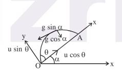
Taking x-axis along inclined plane and y-axis perepndicular to it at point O.
